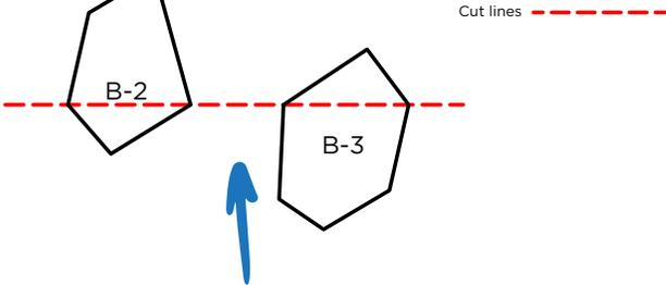
Cut these stones point-to-point for the base start / straight edge.
