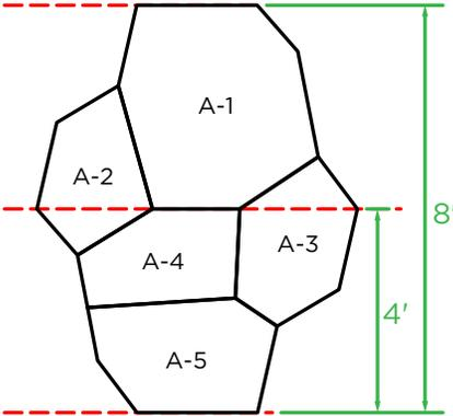
Cut these stones point-to-point for the base start / straight edge.
